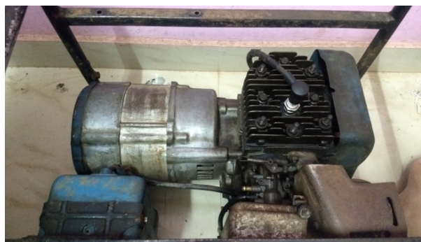
Fig.5. engine connected to alternator
